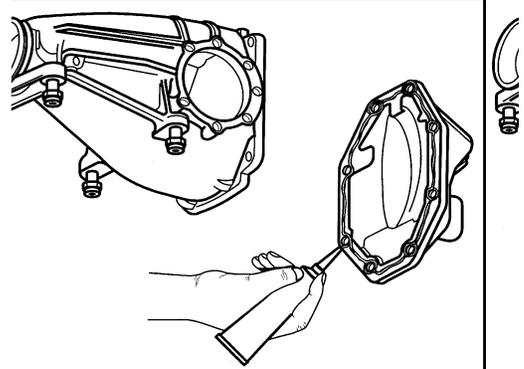
6. Assemble parts immediately while silicone is still wet.
